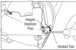
**2.** Release the other end of the spring from the waste bin section. Repeat this procedure on the other end of the cartridge.
