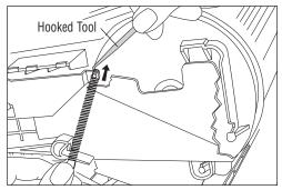
**3.** Attach a new spring to one end of the waste bin section.
