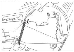
4. Carefully stretch the spring and attach it to the hopper stabilizer post on the hopper section. Be careful not to overstretch the spring. Repeat this procedure on the other end of the cartridge.
