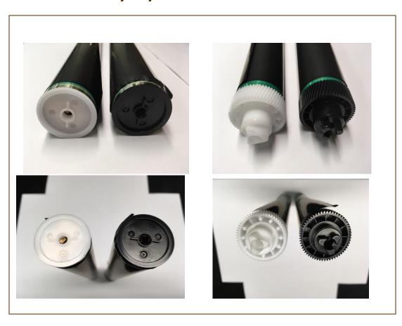
Drum gear change, from black gear to a white gear. This change can be referenced by the photographs shown above. This change does not affect product performance. Mixed shipments are possible. Affected Product Code & Starting Lot Numbers below:
