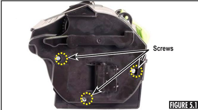
Using a #2 Phillips screwdriver, remove the three screws from the drive side end plate (Figure 5.1) and remove the end plate.
