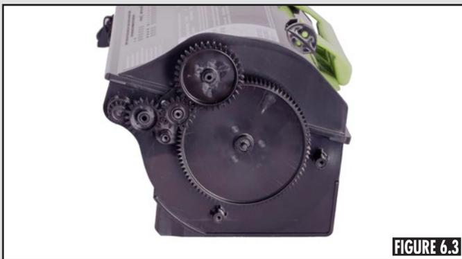
Ensure the drive gears are installed as shown in Figure 6.3.
