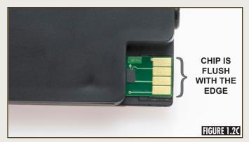
Note: The new Static Control chip should lie flat and be aligned flush with the edge of the cartridge when installed properly (Figure 1.2C).
