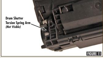
Release the shutter torsion arm from the indent on the drum plate (Figure 11). Open and close the drum shutter to ensure the spring is engaged.
