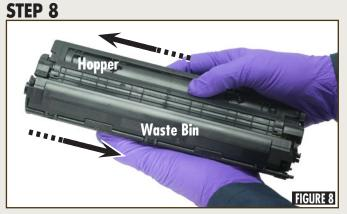
Align bosses on the hopper to openings on the Static Control waste bin. Carefully slide the toner hopper and waste bin sections together as shown in Figure 8. Verify the springs between the hopper and waste bin are straight.
