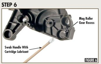
Using a lint-free swab, apply a small amount of cartridge lubricant to the mag roller gear recess on the new Static Control gear side end plate (Figure 6).
