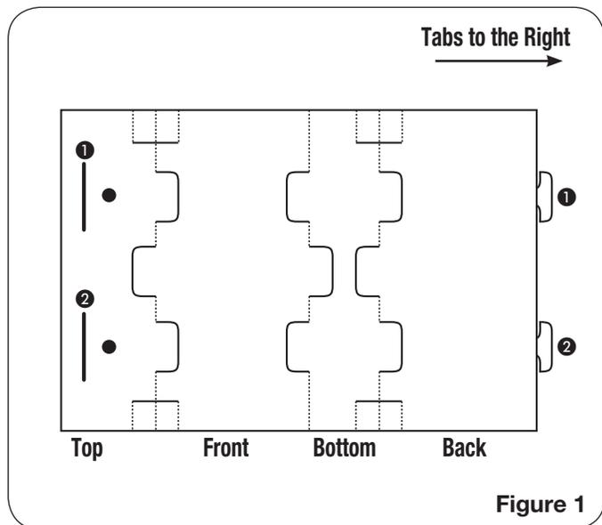
2. Fold up sides and insert tabs (1,2) into corresponding slots and open them to lock the insert (Figure 2).
