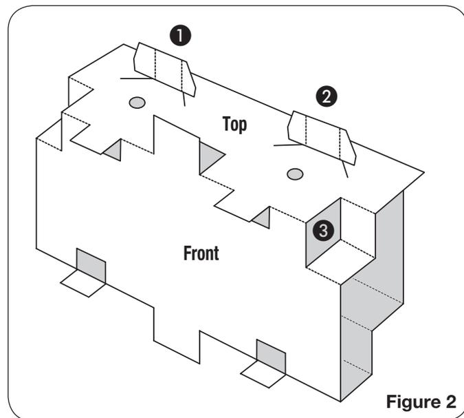
3. Push corners in (3) to lock cartridge into insert (Figure 2).
