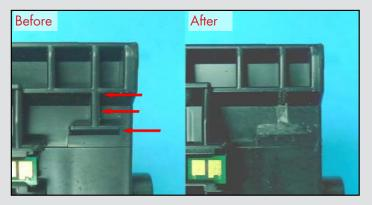
Remove the ribs on the left of the Toner Waste Bin as shown in the photo.
