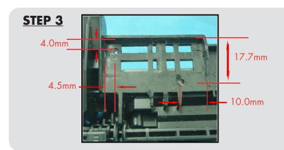
Drill two 2.4mm diameter holes on the cleared platform as shown in the photo.
