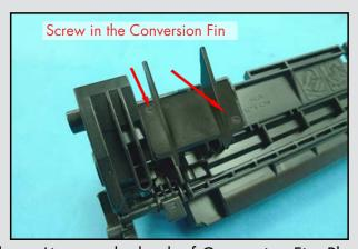
Remove the Release Liner on the back of Conversion Fin. Place the Static Control HM507CONVFIN Conversion Fin onto the platform of the Toner Waste Bin. Then use the screws which come with the HM507CONVFIN to fix the Conversion Fin to the Toner Waste Bin as shown in the photo.
