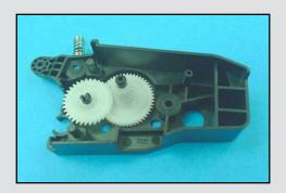
Unscrew the OEM Right End Cap from the Toner Hopper and keep the screws for reuse. Take off two gears from OEM Right End Cap and place them on one side.
