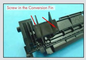
Remove the Release Liner on the back of the Conversion Fin. Place the Static Control HM404CONVFIN Conversion Fin onto the platform of the Toner Waste Bin. Then use the screws which came with the HM404CONVFIN to attach the Conversion Fin to the Toner Waste Bin as shown in the photo.
