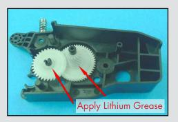
Take the two gears that were set aside & put them back inside the OEM Right End Cap to the corresponding position as shown in the photo.
