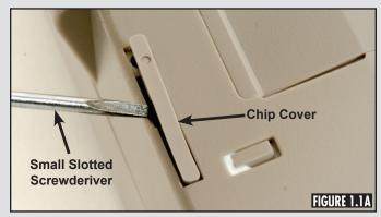
Locate the chip cover on the cartridge. Using a small slotted screwdriver, carefully pry the chip cover up and remove from the cartridge. See Figures 1.1A & 1.1B.
