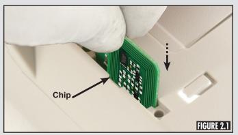
Align the replacement chip as shown in Figure 2.1 and drop it into the chip's slot.
