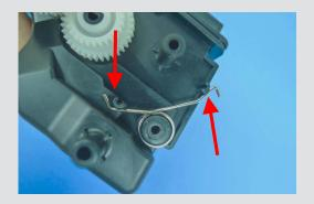
Place the Spring from STATIC CONTROL B9310UHYFGR-10 onto the boss on the cartridge and position the front end and back end of the spring hooked to the two ribs of the cartridge respectively as shown in the photo.
