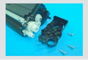
Unscrew the OEM Left End Cap from the Starter Toner Cartridge. Keep the end cap and small screws for reuse.
