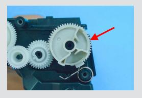
\*\*It is important that after the spring has released, the flag gear is positioned exactly as shown in the photo.
