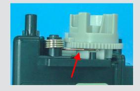
Keep the flag gear in the correct position and then release the back end of the spring from the rib onto the back of the flag gear as shown in the photo.
