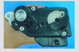
Install the OEM End Cap and install the three screws, making sure the position of the flag gear does not move. If the lever does move, steps 2 to 5 must be repeated. If the flag gear is not in the correct position, inserting the cartridge will not reset the printer.
