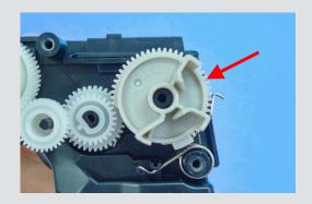
Install the Ultra High Yield Flag Gear from STATIC CONTROL B9310UHYFGR-10 on the boss of the cartridge. Make sure the flag gear is placed at the correct angle as shown in the photo.
