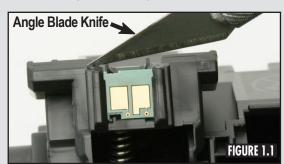
Use the angle blade knife tool and carefully break away the molding covering the top two corners of the spent chip (Figure 1.1).
