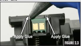
Apply a very small amount of hot glue to the top two corners of the chip to secure the chip in the cartridge (Figure 2.3).
