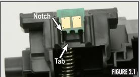
Position the Static Control replacement chip such that the notch is aligned with the tab as shown in Figure 2.1.
