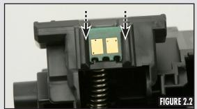
Slide the chip into the cartridge (Figure 2.2).
