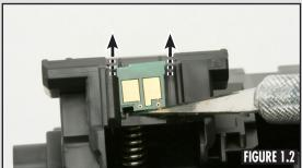
Use the angle blade knife tool and lift the Spent chip out of the cartridge (Figure 1.2).
