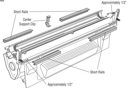
**2.** Use your thumb to press the rail in place. Position the short leg of the rail on the bottom of the flange and roll the rail up and over it.
