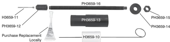
**Kit contains:** 1-Epoxy Applicator with Guide, 1-Epoxy Electrode Applicator and Extractor Assembly (one time use electrode applicator pin, end nut, threaded shaft, guide, washer and jam nut), 1-sampler tube of bonding material (Loctite® #680). Optional replacement adhesive use Loctite No. 638 or Loctite No. 426.
