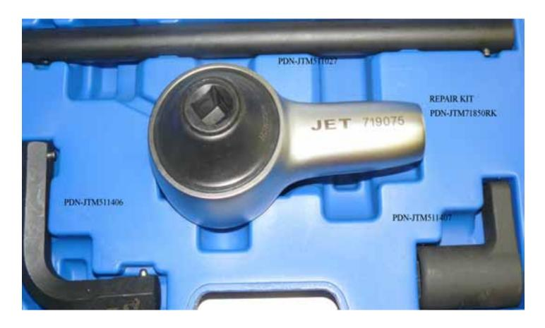
TORQ MULTPLIER REPAIR KITS CONTAIN SUN GEAR AND PLANETARY GEARS
