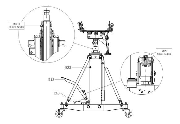
Please follow the instructions to eliminate the air in the pump core if the product is lifting slowly or can't lift up.
