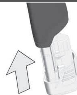
Remove the battery pack before starting any work on the machine.
