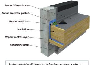
Protan provides different standardised parapet systems.
