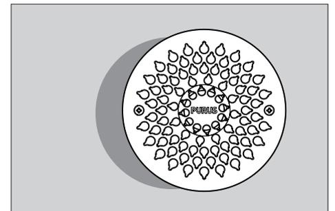
**Note!** Do not unscrew the screws completely. If you do, the nuts will fall into the floor gully. Carefully lift up the grating using a screwdriver.
