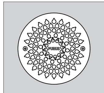
Press the grating into the gully until you hear a click, and tighten the screws.
