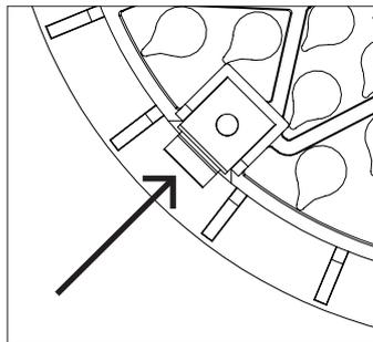
On the underside there is space for two nuts. Affix the square nuts with their beveling facing outwards. The clip on the grating will move outwards when the screw is tightened and presses the grating against the gully's clamping ring.
