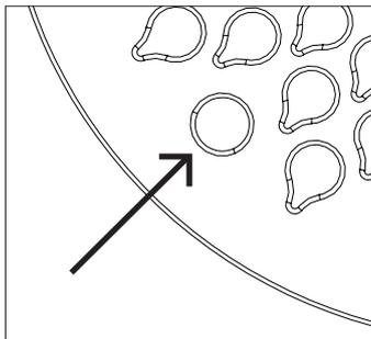
On the upper side of the grating there are two holes for screws.
