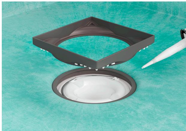
After fitting the waterproofing membrane, it is important to place the 13 mm high plastic frame according to the desired orientation of the surface layer.
