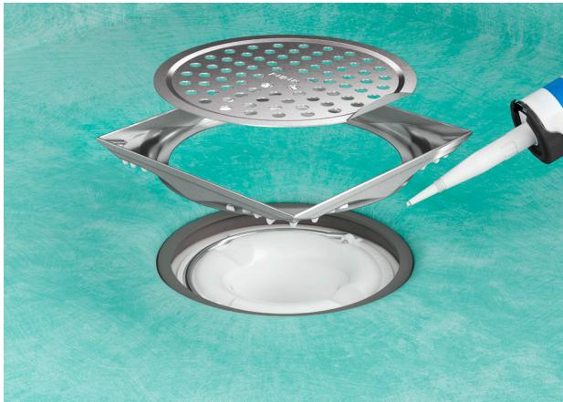
After installing the waterproofing membrane, it is important to position the frame according to the desired direction of the surface layer. The frame is positioned centrally above the clamping ring, make sure that the water trap can be lifted out. The frame must then be spot glued with construction adhesive on the underside to be attached to the waterproofing membrane.
