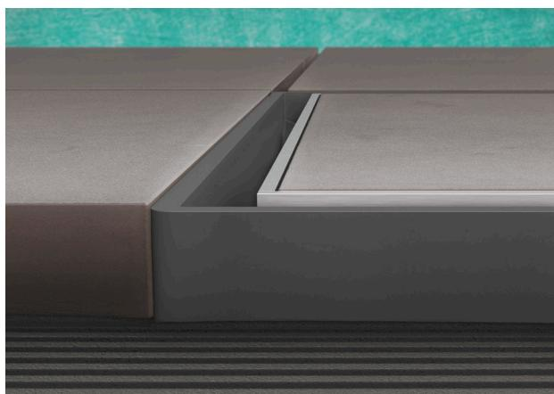
The end result should look like the picture on the left. The plastic frame must be put against the waterproofing membrane and at the same height as the tile/natural stone.
