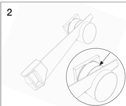
The upper part of the gully can be cut to 85-120mm. Keeping the cut below the marking on the top part. Clear the cut from degrees and such.
