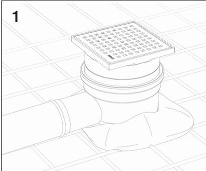
The floor gully must be mounted in a suitable and stable way for a horizontal installation and installed in a way that makes it possible to clean and remove the water trap.
