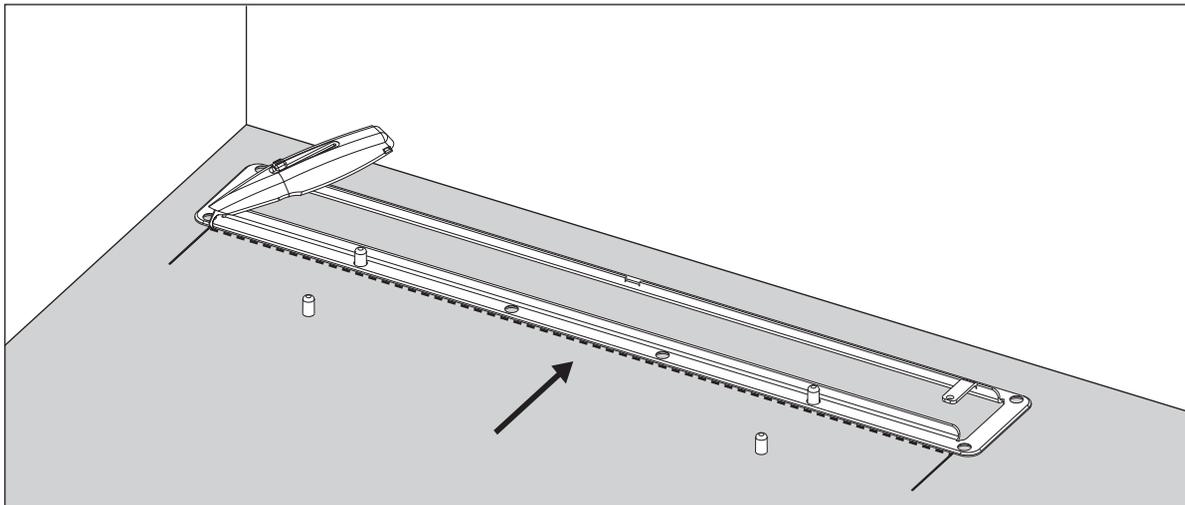
Move the frame and place it over two of the guide sleeves, and then cut along the outer edge of the long side like a ruler.
