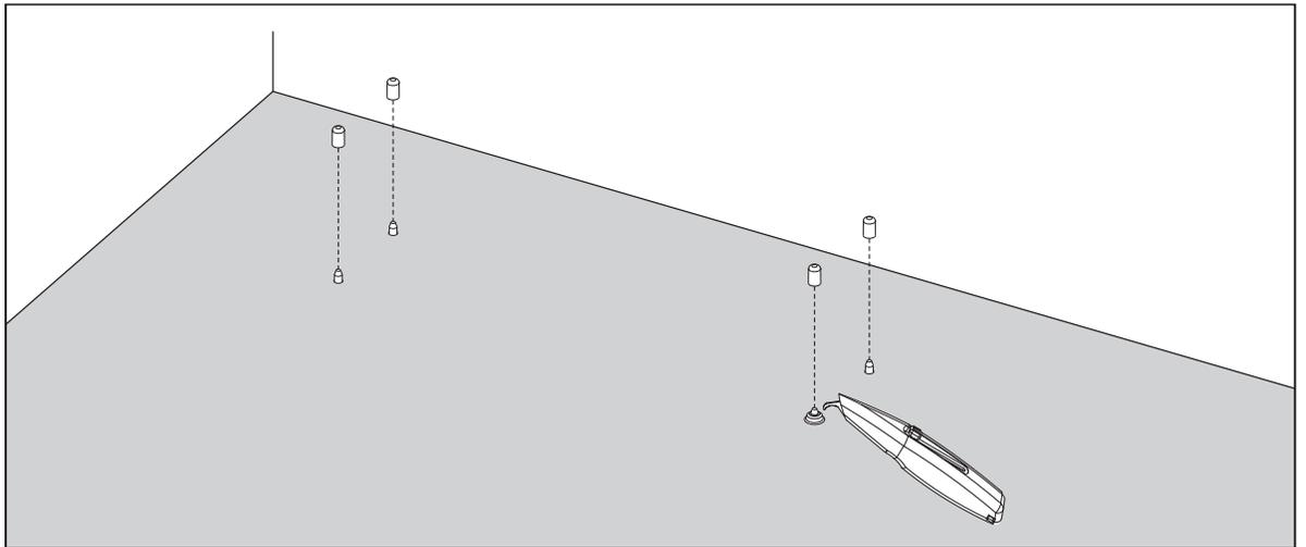
Lay out the vinyl flooring sheet and press down so that the studs of the cutting template cut through. Make sure the studs are clear of the vinyl sheet all the way down. Then place the guide sleeves on the studs.
