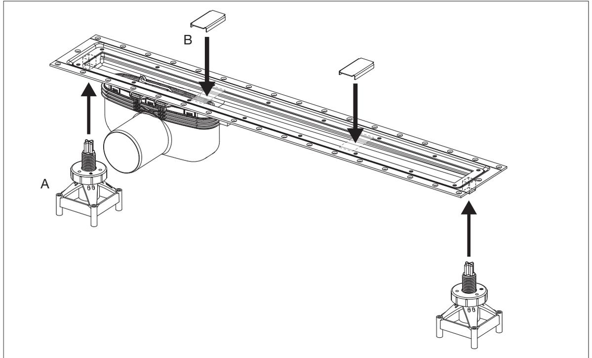
Underneath the floor gully are fasteners for the Purus supporting legs. Press the Purus supporting legs into place and adjust to the desired height (A). Place the mounting plates in the channel drain to prevent it becoming deformed when the concrete is cast (B).
