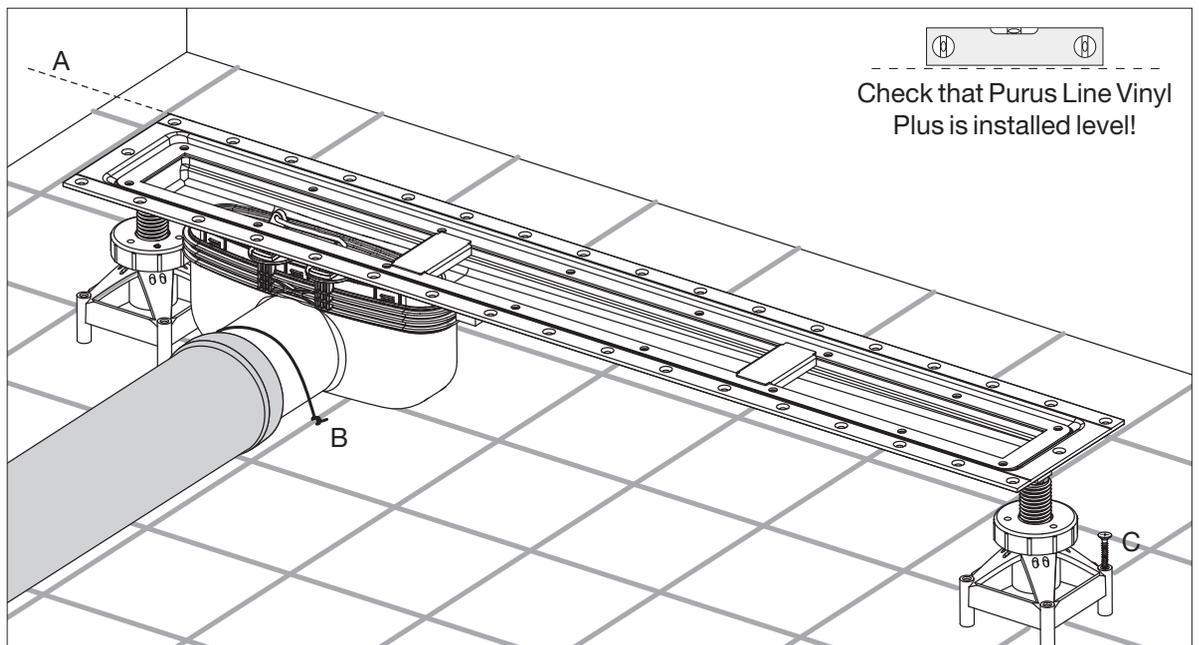
Position Purus Line Vinyl Plus with the upper edge level with the finished floor, i.e. level with the vinyl flooring.
