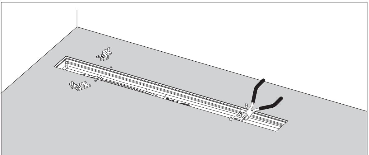
Remove the frame, the guide sleeves and the cut-out section from the vinyl sheet. Split the cutting template and remove.
