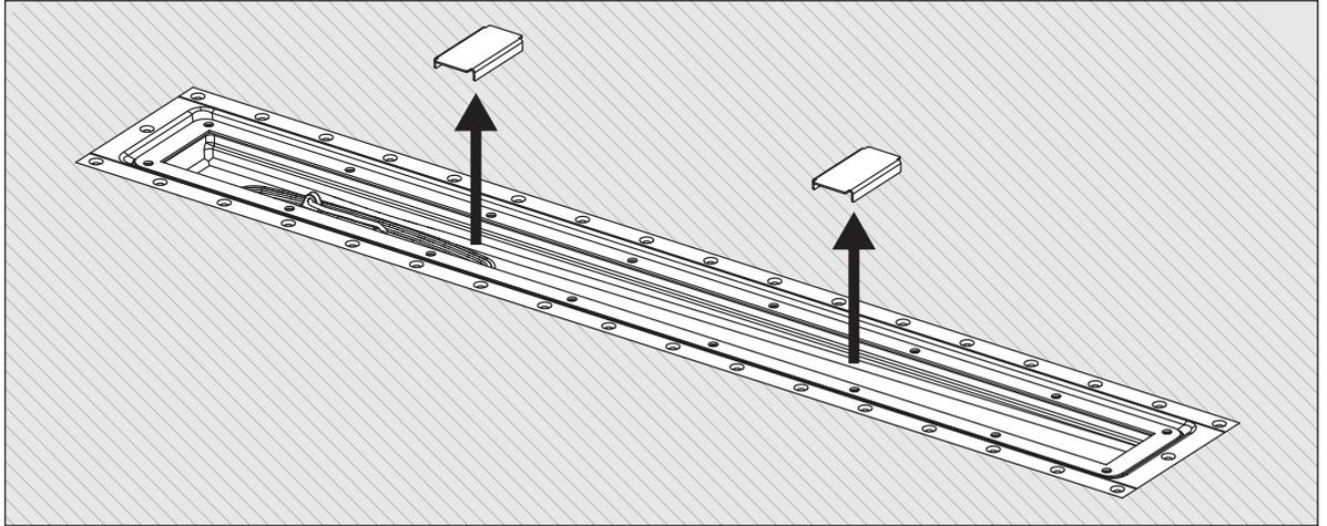
Screed the floor. Remove the mounting plates.
