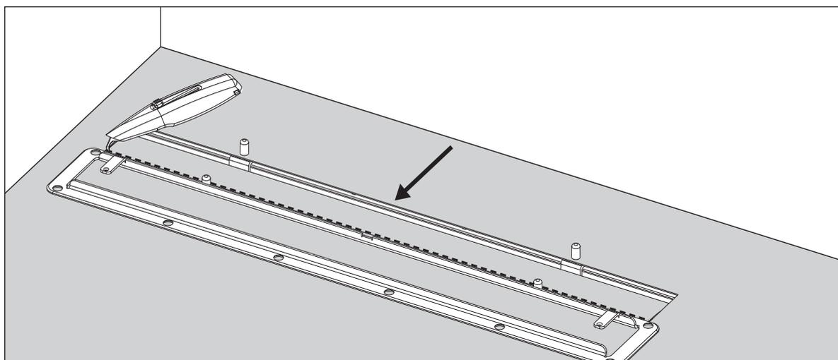
Move the frame and lay on the opposite side of the other two guide sleeves and then cut along the outer edge of the other long side like a ruler.
