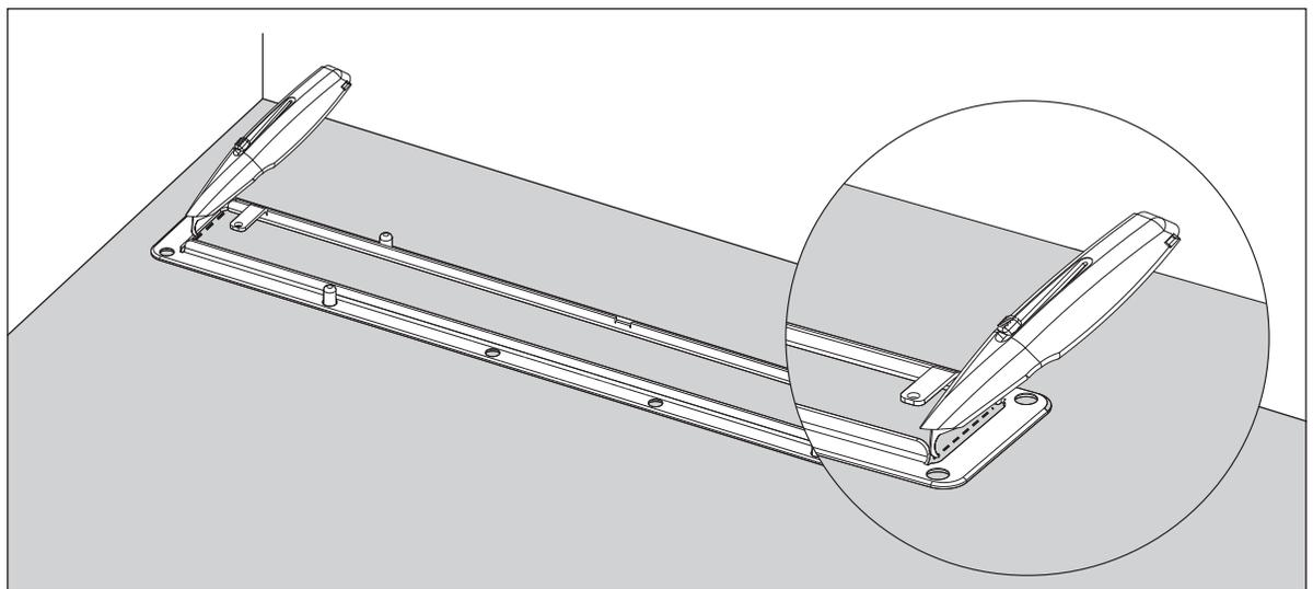
Place the frame upside down on the four guide sleeves. Only cut the edges on the inside of the frame.
