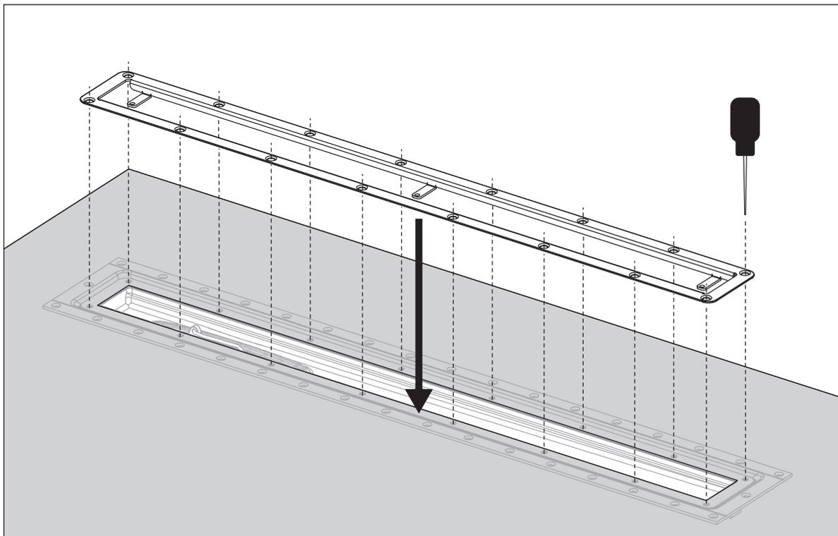
Lay the clamping frame in place and make holes for the screws with an awl or similar.
