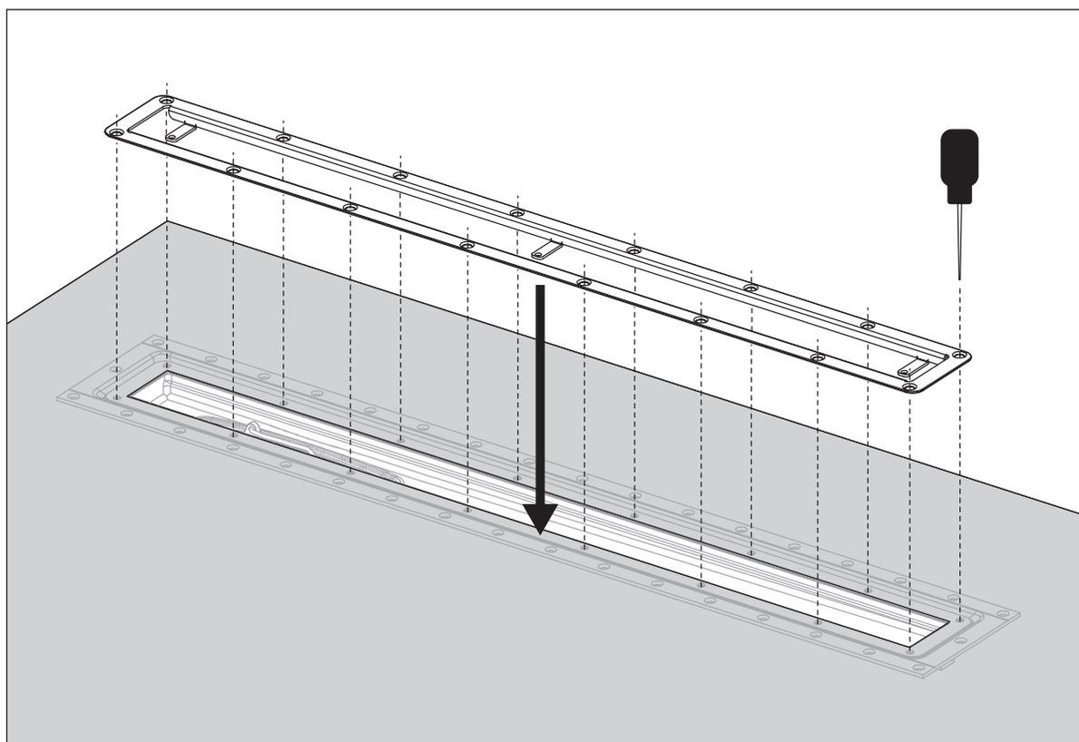
Lay the clamping frame in place and make holes for the screws with an awl or similar.
