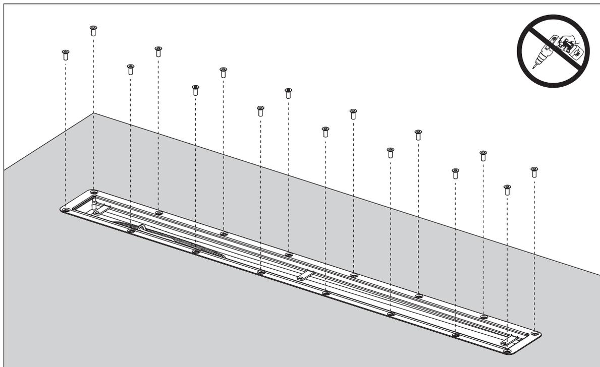
Reheat the flooring if necessary. Firstly, fix the screws loosely in each screw hole. Then tighten the screws by hand in stages, beginning with the middle of the clamping frame working outwards until they are screwed all the way in. Use hand tools!
