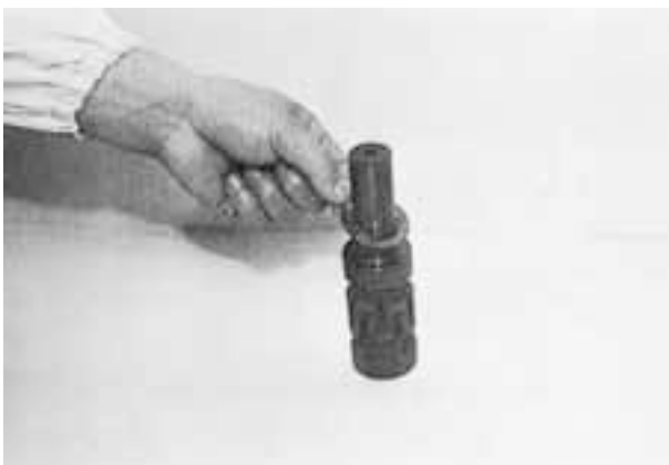
(10) Take out needle bearing from output shaft.
