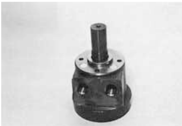
(3) Install output shaft in housing.
