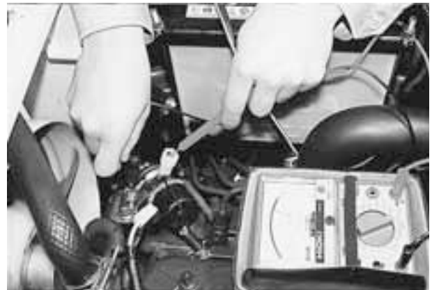
Check conductivity between the solenoid terminal and the body ground. (Photo 6)
