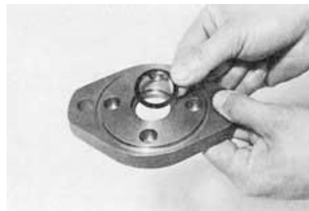
(4) Fit dust seal in flange. Use appropriate jig not to damage seal or distort metal plate. Apply hydraulic oil on outer side of seal. Fit seal on flange and press fit. This seal contains metal plate in rubber. Case should be taken ont to damage seal or distort metal plate.
