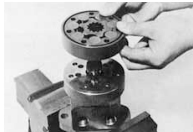
(15) Install geroler. Care should be taken on the position of output shaft, geroler and geroler set. Refer to the figure below.
