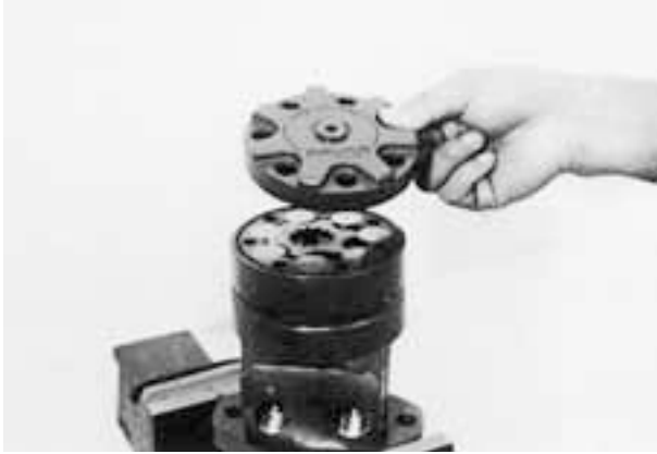
(17) Put end cap onto geroler set, aligning to bolt holes.
