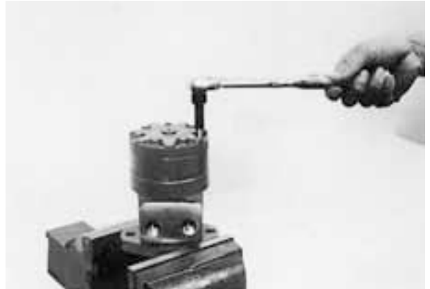
(18) Tighten 7 pieces of end cap mounting bolts. Model S-380 requires screw locktite #262.
