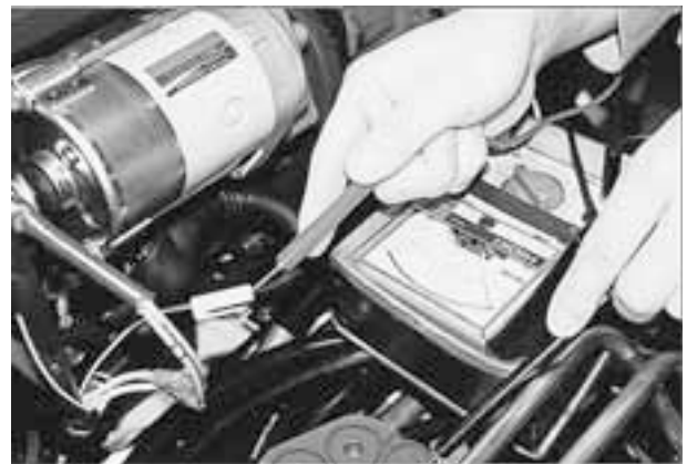
2. Is battery voltage applied to the self-starting motor in starter switch ON position? (Photo 4)
