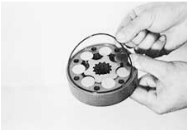
(14) Fit O-ring (2 pieces) onto geroler. Apply grease on O-ring and securely fit.
