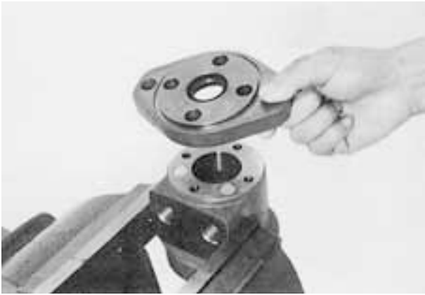
(12) Take out flange. In case of S-280 and S-380, 4 pieces of spring pins are installed, Therefore, remove flange by slightly tapping the flange by plastic hammer, then pull out spring pins.
