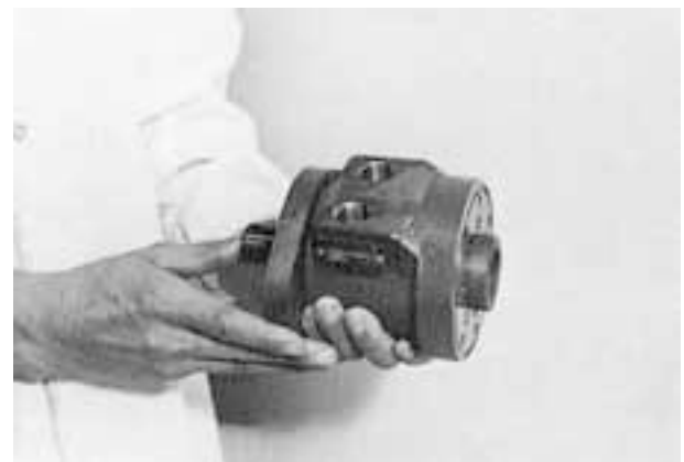
(9) Dismount motor from vise and push out output shaft.
