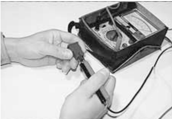
1. Checking slow-low fuse for breakage (Photo 3)
