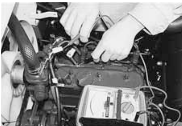
Is voltage applied for about 10 sec. when the starter switch is OFF? (Photo 3)
