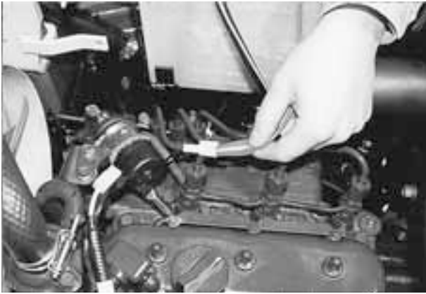
Apply battery voltage to the engine stop solenoid and check to see whether or not the injection rubber is drawn in and the rack bar returns when the application of voltage is stopped. (Photo 5)
