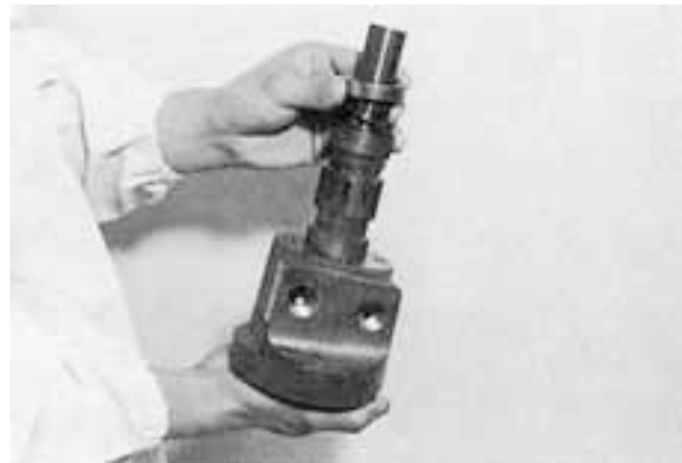
(3) Insert needle bearing and bearing race into output shaft.
