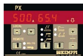
PX control panel
