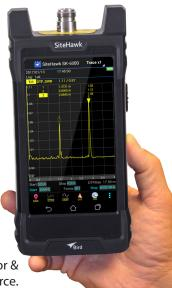
Locate RF cable, connector & antenna problems at the source.
