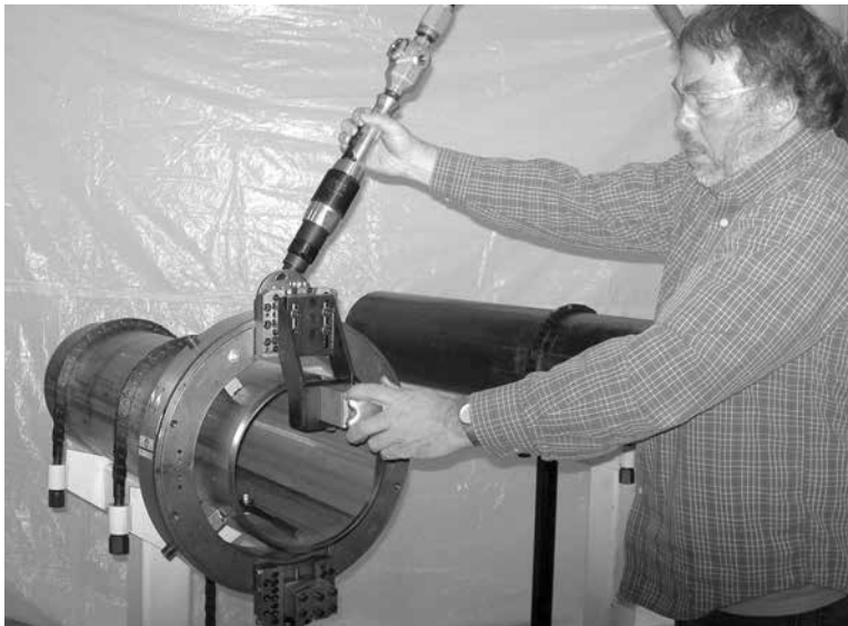
Figure 2-9. When using accessories that require you to operate their controls (shown with universal counterbore slide), stand in a position where you can operate the machine without contacting moving parts.
