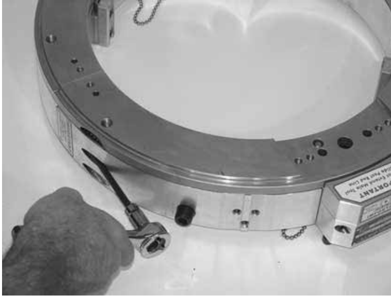
Figure 5-16. Loosen the captivated screws to separate the halves.
