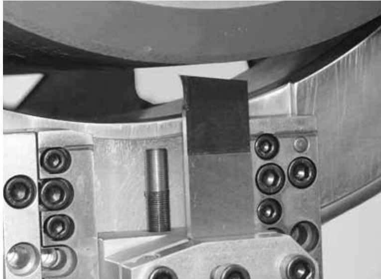
Figure 5-37. Set the tip of the parting tool 1/8" (3 mm) from the pipe surface.
