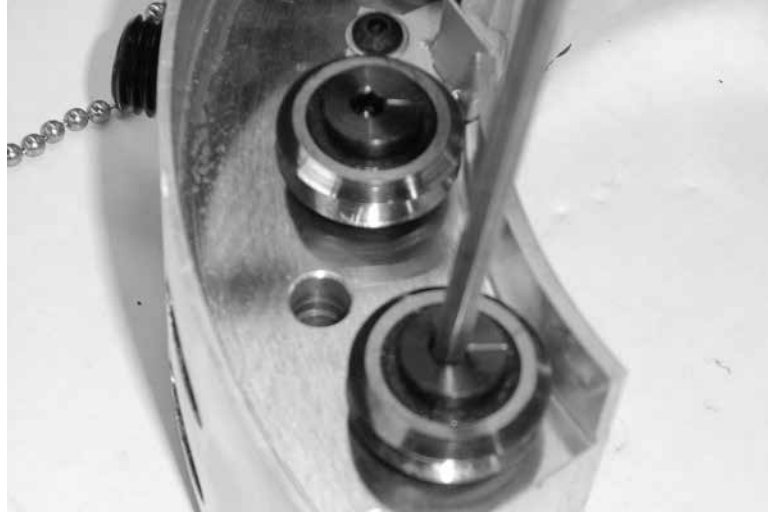
Figure 7-16. Set the marks on the eccentric shafts toward the center of the ring.
