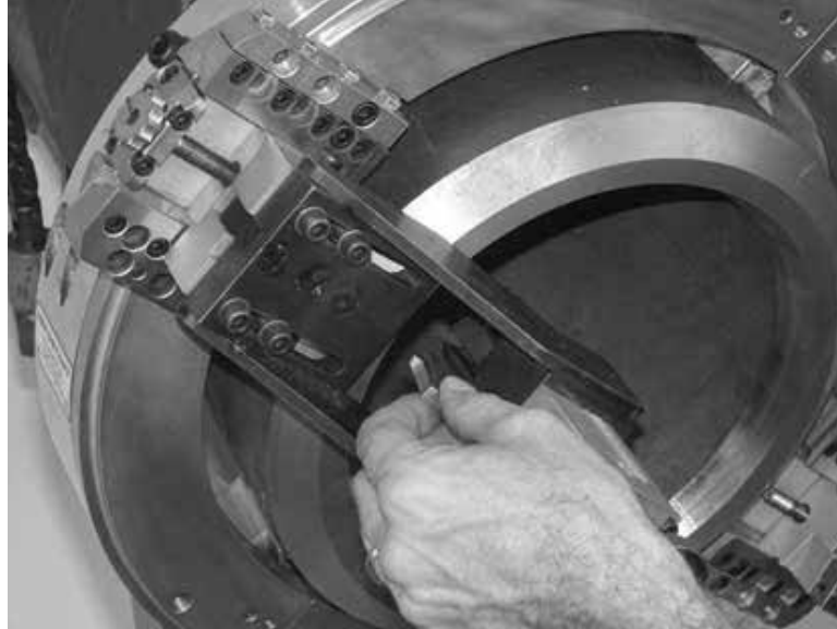
Figure 5-65. Install the counterbore tool into the slot.
