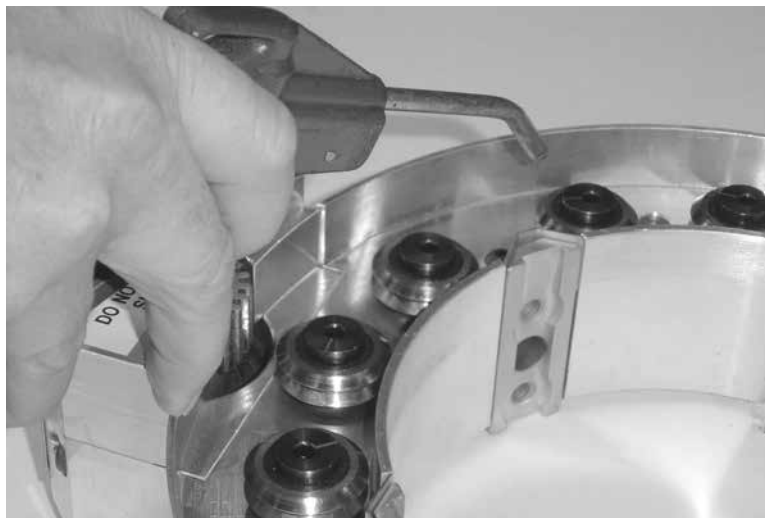
Figure 7-12. Clean debris from the stationary ring.
