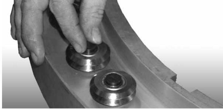
Figure 7-5. Rotate the eccentric shafts so that the high point of each bearing faces the inside of the ring.
