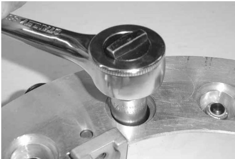
Figure 7-15. Loosen the lock nuts.
