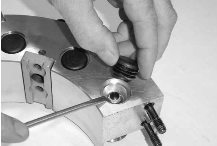
Figure 7-14. Remove the plastic caps to inspect the bearing assemblies.
