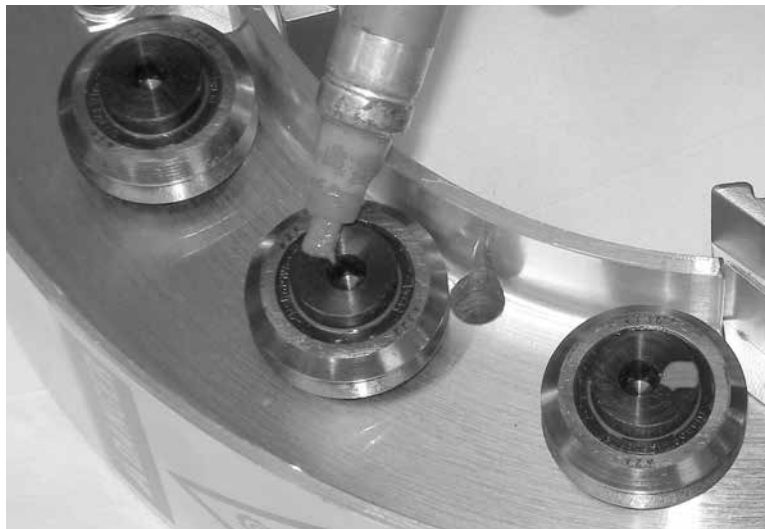
Figure 7-4. Mark the edge of each bearing.
