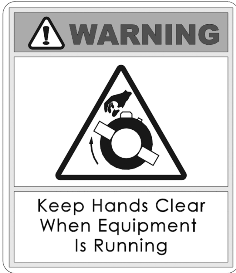
Figure 2-19. The “Keep Hands Clear” label is attached to the stationary ring of the LCSF. Stay clear of moving parts when the LCSF is operating. (Part no. 60-363-00.)
