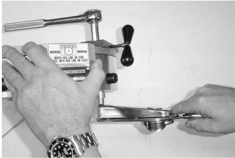
Figure 7-20. Secure the eccentric shaft.
