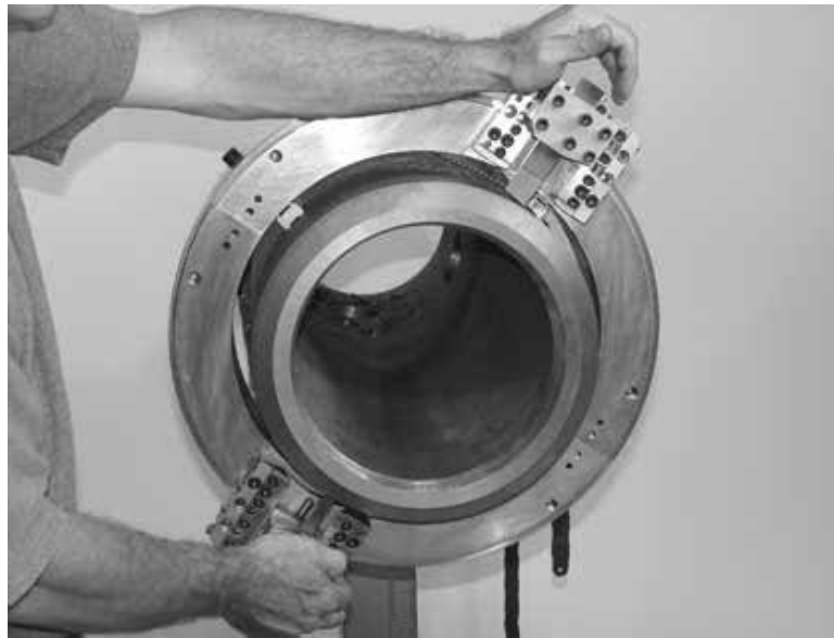
Figure 5-34. Rotate the machine to check tool clearances.
