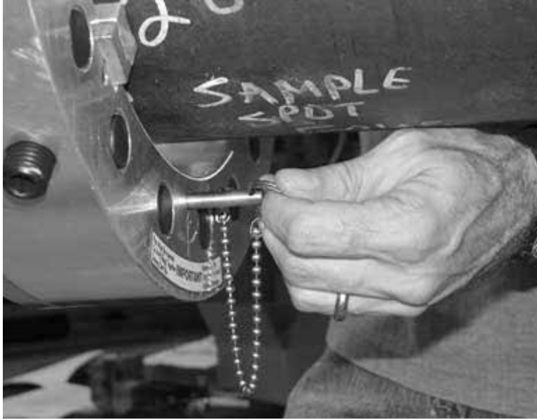
Figure 5-25. Remove the frame locking pins.
