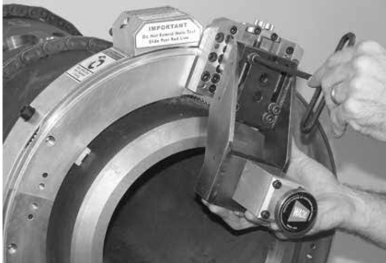
Figure 5-63. Attach the counterbore slide.
