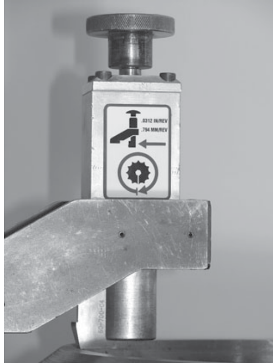
Figure 5-69. Axial (.0312) and radial (.0784) adjustment per revolution
