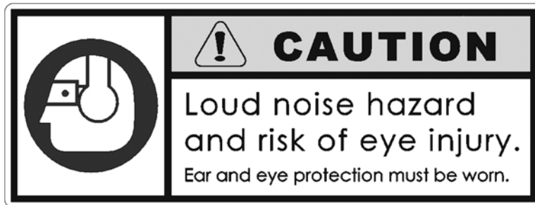
Figure 2-14. The ear and eye protection label is attached to the drive motor of the LCSF. Always wear ear and eye protection when operating the equipment. (Part no. 90-401-03.)
