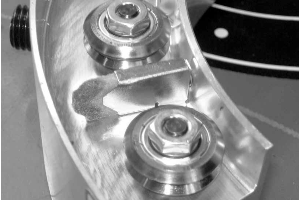
Figure 6-3. Turn the rotating ring out of the stationary ring far enough to access the wipers.
