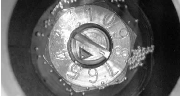
Figure 6-1. Use the needle valve screw to adjust the drip rate of the air motor oiler.
