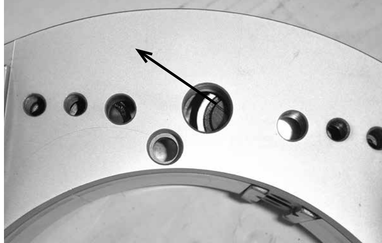
Figure 7-22. Check for bearing rotation as you turn the rotating ring.
