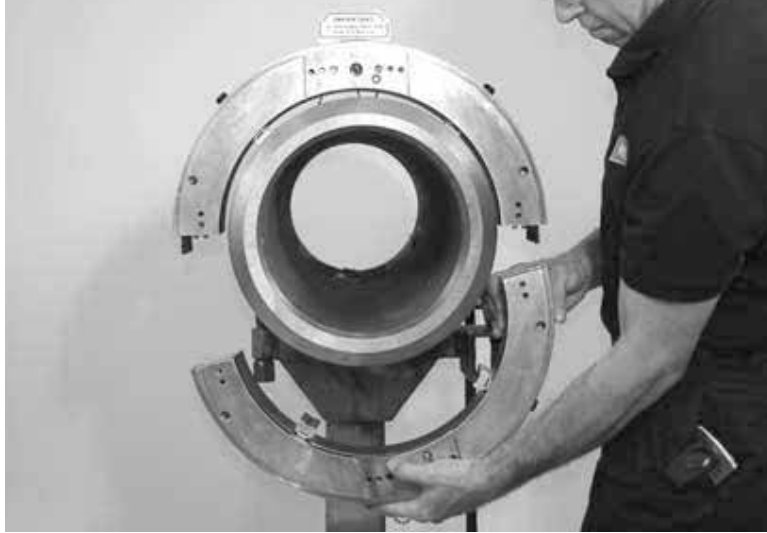
Figure 5-19. Fit the halves together on the pipe.
