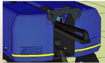
■ PULL-OUT CABLE SYSTEM Internal hoses and cables can be pulled out by cartridge
