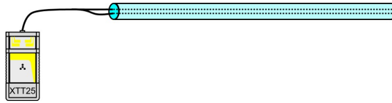
Figure 5.2.a. Transmission should always be connected to a pair: If the output is transmitted to wires of a different pair or wires located in different quads, cross talk with other wires will result.
