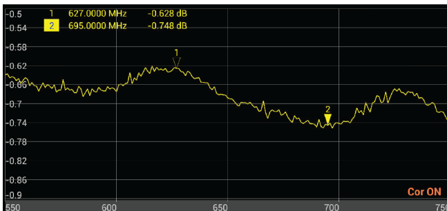
Figure 11 Interpreting Cable Loss Measurement
