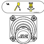
**NOTE:** Main lift and swing functions may be selected at the same time. Maximum speed is reduced when both functions are selected.
