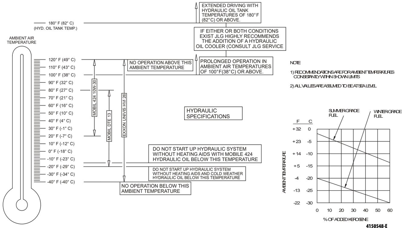
Figure 7-2. Engine Operating Temperature Specifications - Deutz 2.3L - Sheet 2 of 2
