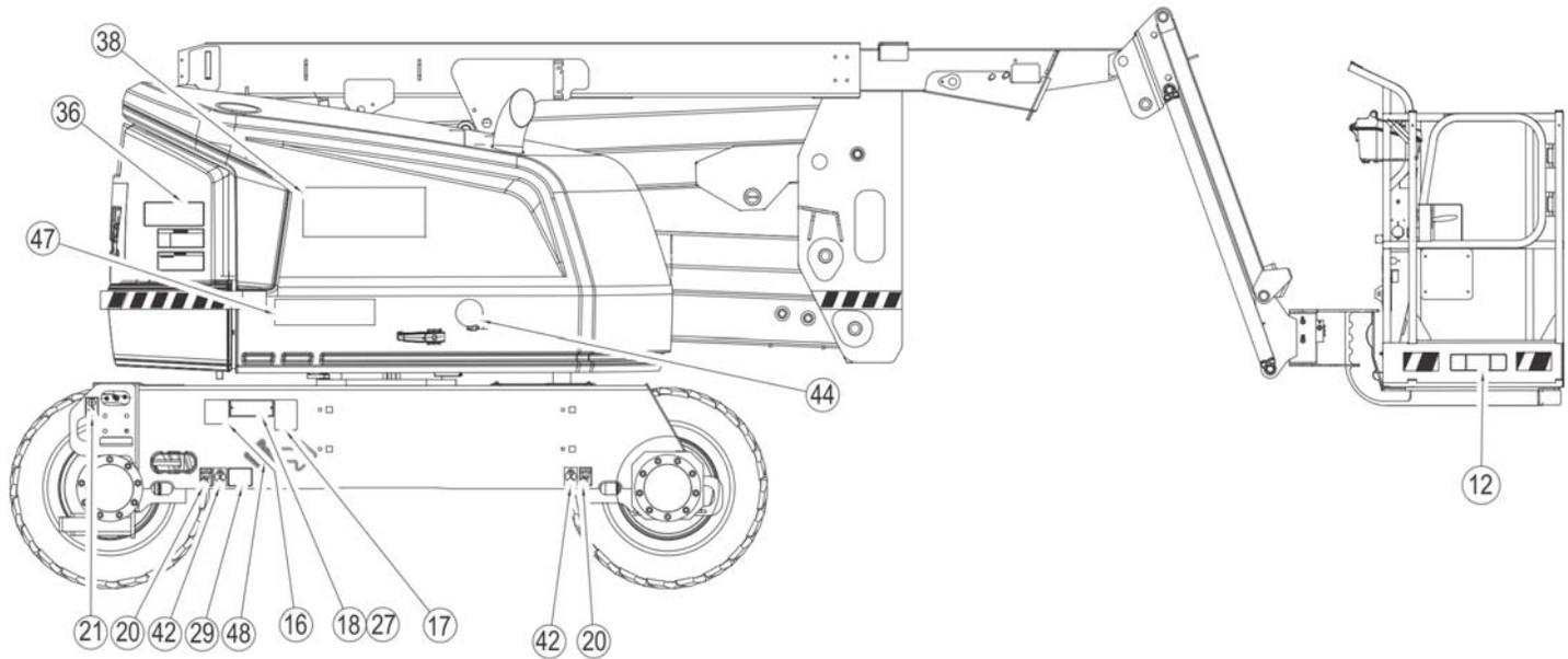
Figure 4-6. Decal Location Sheet 1 of 6
