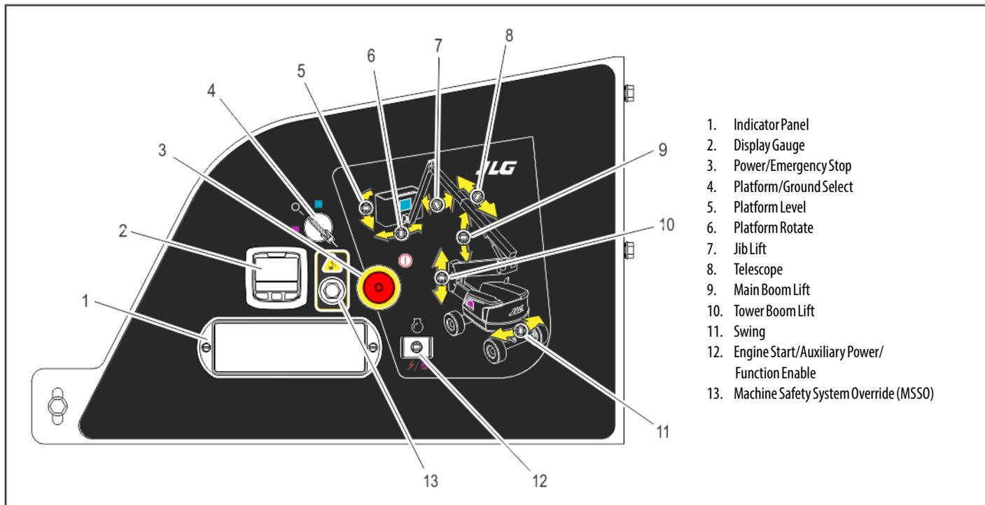
Figure 3-2. Ground Control Console with MSSO (CE Only)
