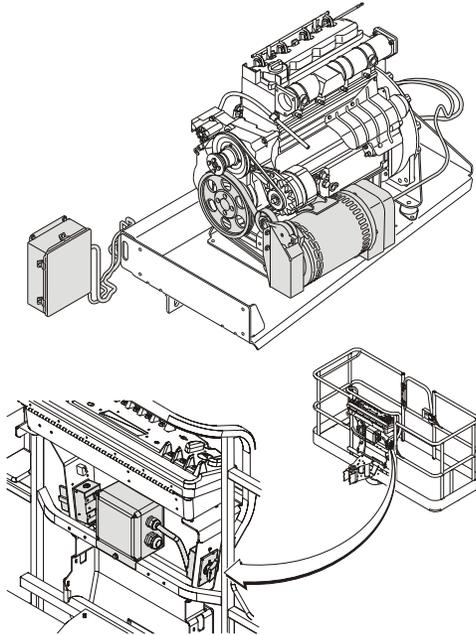
The SkyPower™ system supplies AC power to the platform through an AC receptacle to run tools, lights, cutting, and welding equipment.
