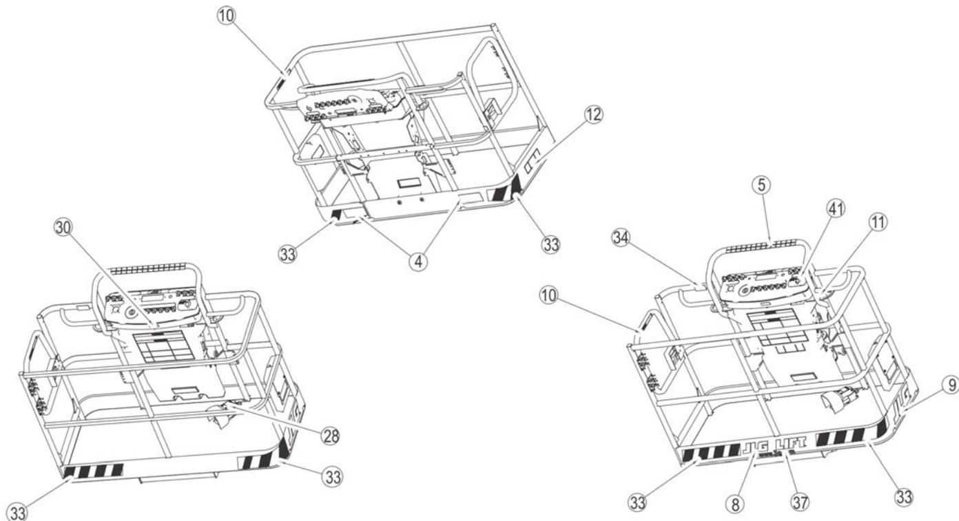
Figure 4-9. Decal Location Sheet 4 of 6
