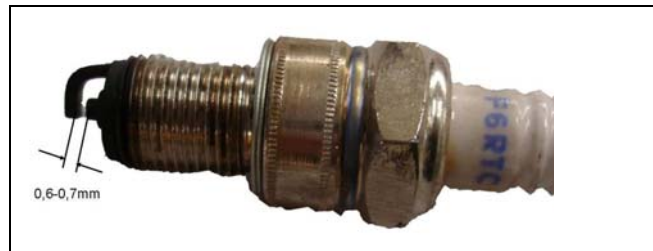
Checking the ignition spark Figure 13: Electrode gap
