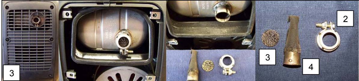
Figure 14: Cleaning the spark catcher
