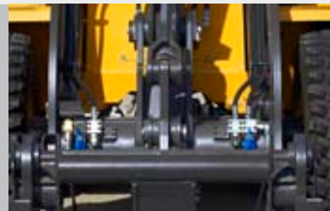
3 rd and 4 th hydraulic circuit
