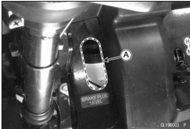
A. Inspection Hole
