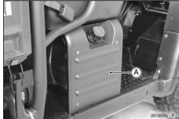
A. Fuel Tank
