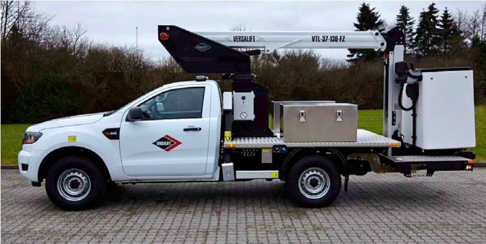
**Length:** 6,625 mm      **Height:** 2,555 mm      **Wheelbase:** 3,220 mm
