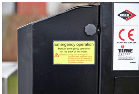
Ground level emergency lowering from the chassis (pedestal mounted valve bank)
