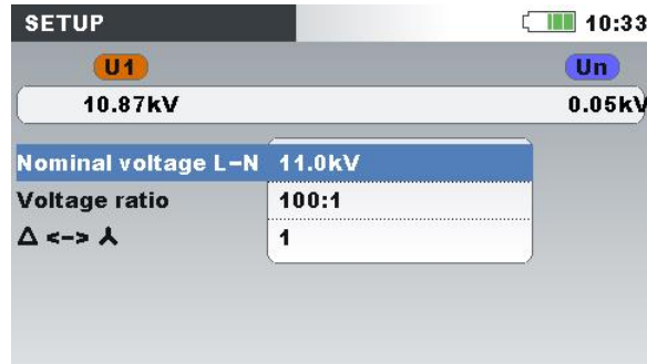
Figure 4.17: Voltage ratio for 11 kV / 110 kV transformer example
