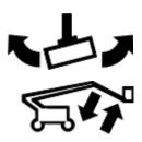
24 Axle extend/retract switch with indicator lights
