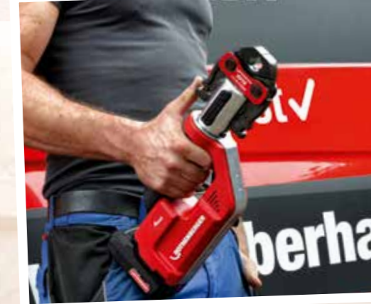
Secondary effect of the two-cylinder-structure: The machine can be used with one hand.
