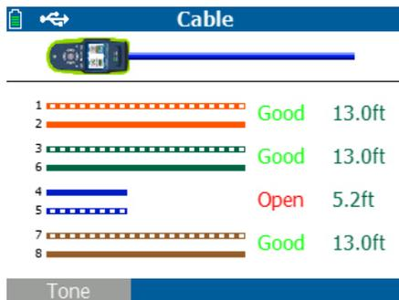
Cable test showing pairs 4 and 5 are open.
