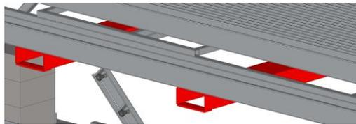
2 Check the height of the platforms and the distance between two platforms
