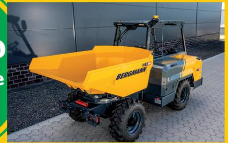
With a payload of up to 3.5 tonnes, the C804e is currently the world's biggest electric wheeled dumper.
