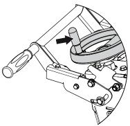
Loosen the screw. Position the indicator arrow to "0".
