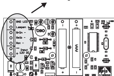
The control PCB is fitted with buffer batteries (cannot be recharged) which maintain the program when changing the main battery.
