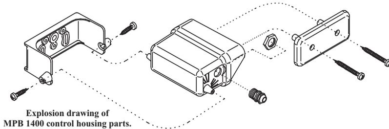
To replace the control PCB, please separate from the operating voltage by disconnecting the batteries in the battery casing. Now disconnect the cable lead from the control PCB to the signal head by simply pulling the plug terminal upwards. This means that you do not have to unscrew the cables. Please pay attention to correct polarity when fitting the new control PCB.
