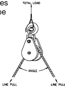
$$\text{The Total Load on the Block} = \text{Line Pull} \times \text{Angle Factor}$$
