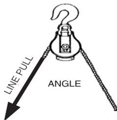
At 0 degrees the multiplier is 2, if the line pull is 1,000 lbs., the total load on the blocks is:
