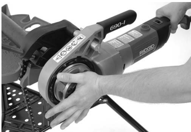
Figure 13 – Entamer le filetage
