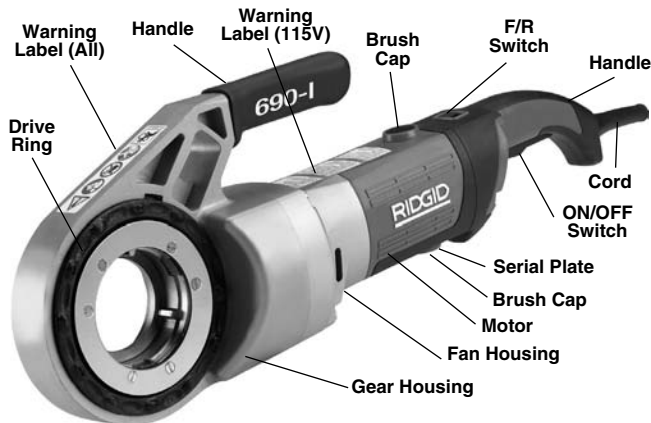
Figure 2 – Model 690-I Power Drive
