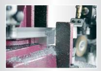
Automatic switch-off after termination of cutting
