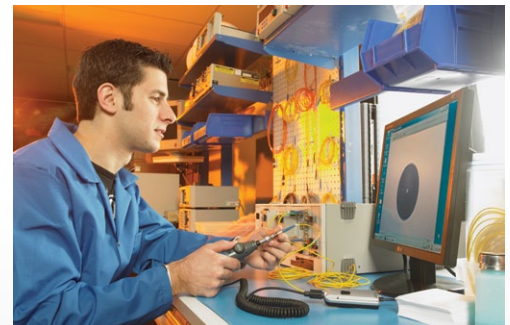
Patchcord inspection in a manufacturing environment
