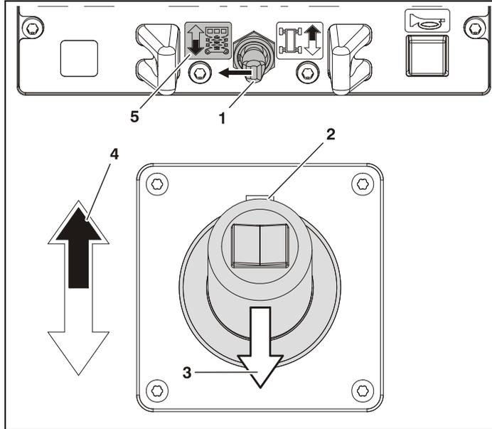
Figure 4-7. Raising Platform From Platform Control
