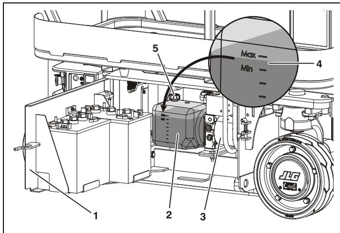
**Figure 6-1. Hydraulic Oil Check Procedure**
