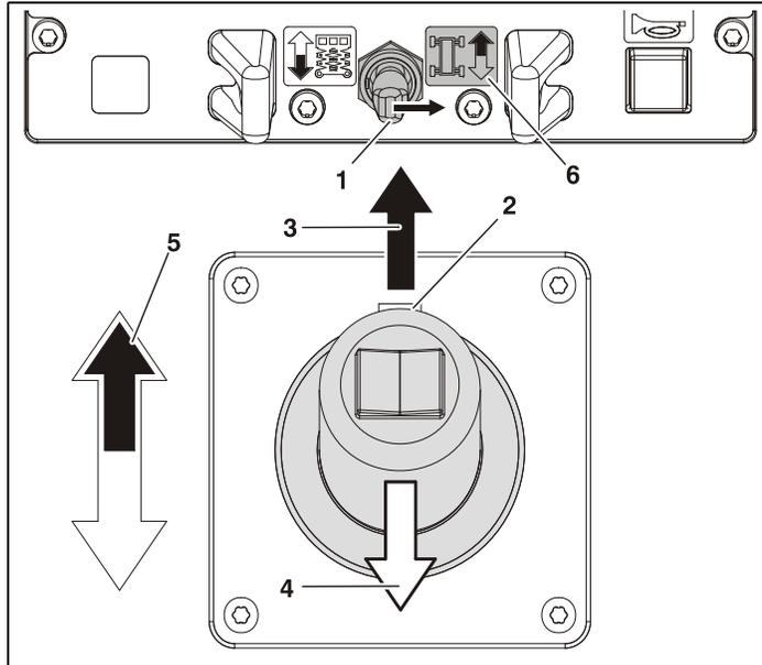
**Figure 4-11. Driving Forward from Platform Control**
