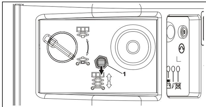
**Figure 4-8. Lowering Platform From Ground Control**
