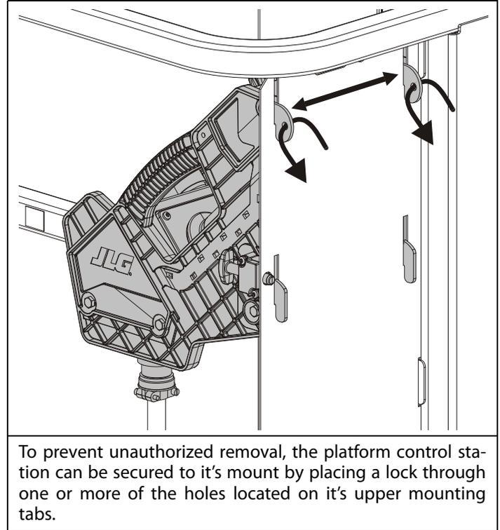
To prevent unauthorized removal, the platform control station can be secured to its mount by placing a lock through one or more of the holes located on its upper mounting tabs.
