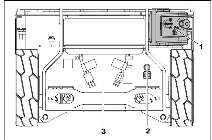
Figure 4-17. Electric Brake Release.
