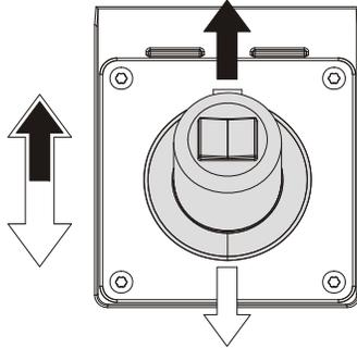
**Drive** - The drive function must be selected using the drive/lift selector switch (*items 5 and 6 on the Platform Control/Indicator panel - Figure 3-8.*), prior to moving the control handle. After selecting the drive function, engage the trigger switch lever, then move the control handle forward to drive the machine forward or move the control handle backwards to drive the machine backward.
