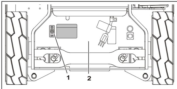
**Figure 4-2. Location of AC Inverter ON/OFF - Toggle Switch**
