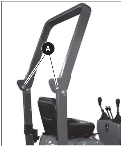
Fig. 82: Lowering the rollbar
