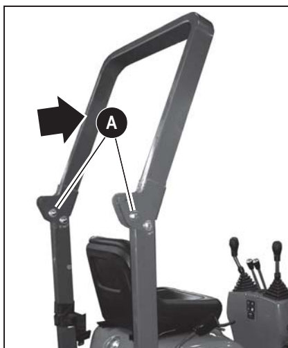
Fig. 84: Raising the rollbar
