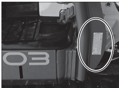
Fig. 2: ROPS bar type label (symbolic representation)
