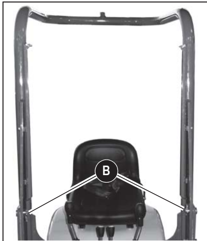
Fig. 86: Lowering the rollbar
