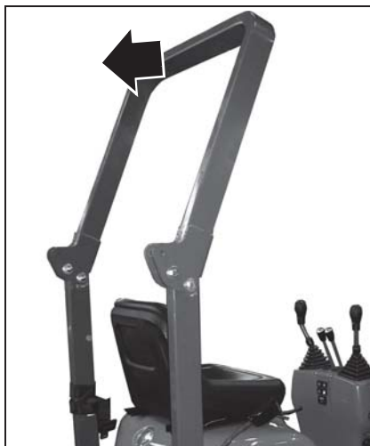
Fig. 83: Lowering the rollbar
