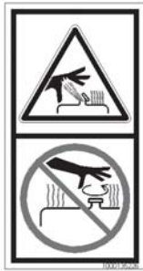
Fig. 26: Reservoir under pressure
