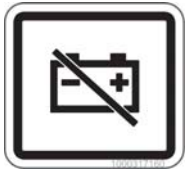
Fig. 21: Battery master switch
