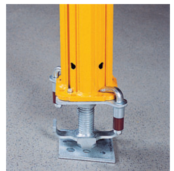
MULTIPROP Tilting Base MKF For use on sloping support surfaces in connection with frames. Tilting in any direction by 3°.
