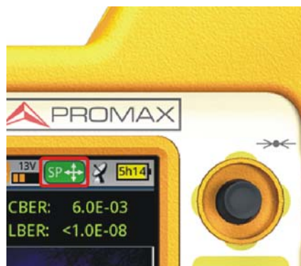
Figure 16. Joystick with SP function enabled (SP: Span)
